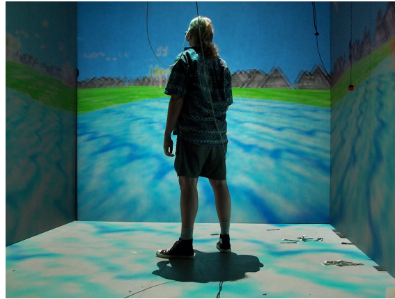
Figure 3.1: Cave automatic virtual environment (picture by Davepape)
